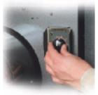
Use the High Idle (OCV) engine speed adjustment dial to change the heat input to the arc:
